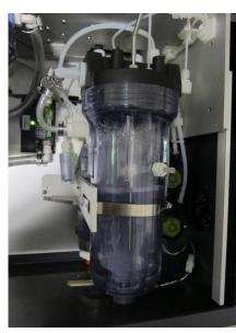
The system have an equilibrator that balances the CO<sub>2</sub> in seawater with a headspace gas that is analysed.
