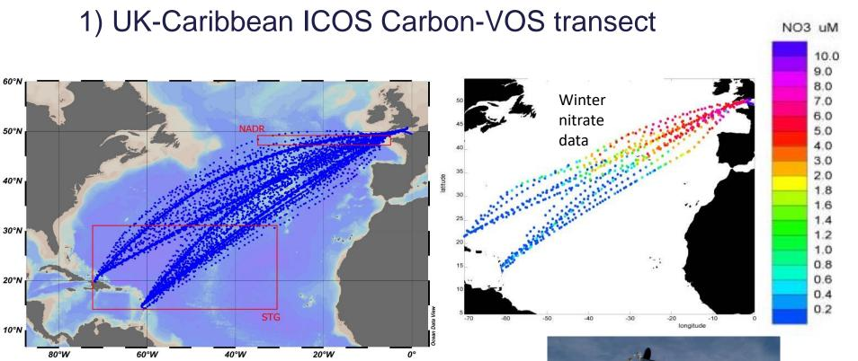
Since 2002 (4 ships) Underway **pCO<sub>2</sub> equilibrator** system, T/S and sampling for nutrients
