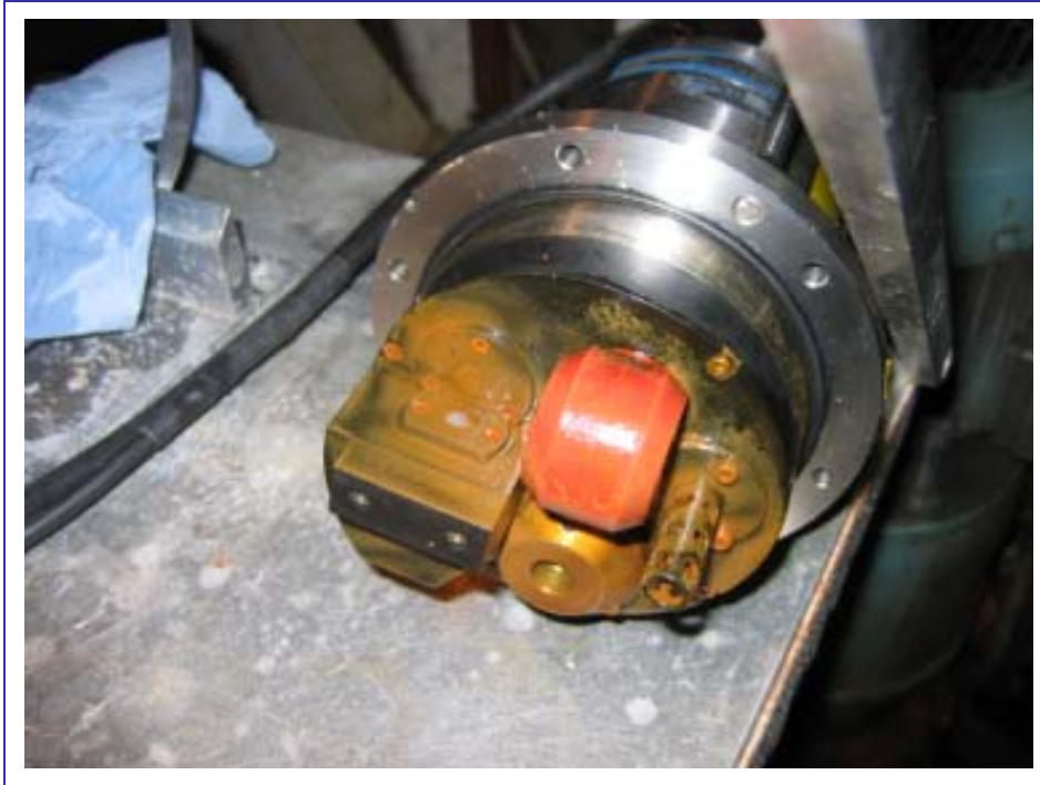
Figure 8-2: Photograph of the CTG MINI pack head immediately after removal from the flow chamber in August 2005 prior to the cleaning.
